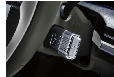
Column-type Shift by Wire (SBW)
