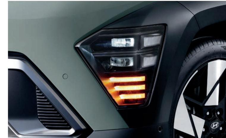
Full LED headlamps (projection type)
